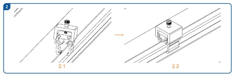
Determine the positions where the clamp will be attached on the roof rib and mark the positioned point. Loosen the one M8\*40 inner hex bolts of the pre-assembled clamp so that the bottom opening of the clamp can become larger. Install the clamp onto the roof rib by an electric wrench or allen key. Install the clamp onto the marked point of the roof rib by an electric wrench or allen key.  $M8 \text{ Torque: } 15 \sim 20 \text{ N} \cdot \text{m}$
