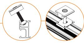
Insert the mid clamp nut by tilting it into the top opening of the rail, then put the second panel onto the rails. Fasten the mid clamps with inner hex bolts M8 at all locations where two panels meet.  $M8\ Torque$ :  $15\sim20N\cdot m$
