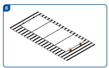
Install all the panels and fasten end clamps at the end of each array. M8 Torque:  $15\sim20N\cdot m$
