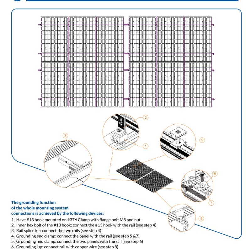
7. Copper wire: connect the mounting system to the ground (see step 8)
