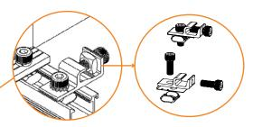
Install a grounding lug onto each rail line edge with an inner hex bolt M8\*25 and a stainless steel nut, then connect 8.4mm² (greater than or equal to 8AWG) copper wire through all the grounding lugs (fixed by M8\*20 inner he x bolt), finally connect a copper wireto the ground. The grounding lug has grounding function when fastened tight to the rail and copper grounding wire. M8 Torque: 15~20N·m
