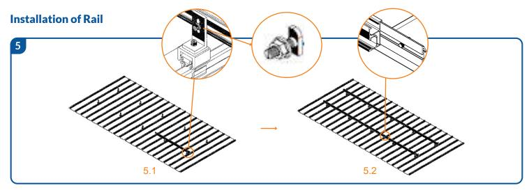
Connect the rail to the 13# hooks with T-bolt and nut. Fasten to secure. Use the rail splice kit to connect the two rails with the two M8\*12 inner hex bolts. The ripple surface of the inner hex bolt, the two bolts and the two star washers of the rail splice kits have grounding function when fastened tight.  $M8 Torque: 15\sim 20N \cdot m$
