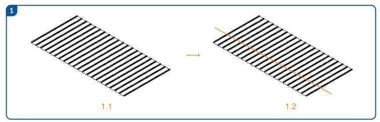
Determine where the roof mounts will be positioned and use a tape measure or chalk line to mark the roof.
