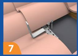
Drive two 3/8"bolts in to the rafter to secure the hook in place
