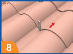
Return the tile to its original location. Slight alteration to the bottom of the tile may be required where the hook protrudes.
