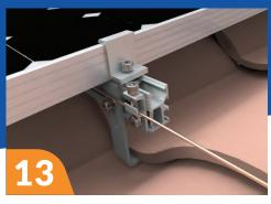
Install the Grounding Lug on each The system is complete. section of rail. Run copper wire to connect them all. Tighten to 3 Ft Lb.
