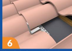
Place the hook on top of the rafter to which it will be installed. Make sure the hook is in contact with the tile below it to prevent damage to the roof.
