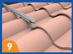
Connect Chiko Solar 'proprietary Railto the hook using a flange nut andbolt. Tighten to secure (18 Ft Lb).
