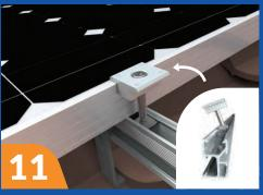
Insert the Mid Clamp nut by tilting it in Insert End Clamp nut by tilting it in the the opening on the top of the rail. opening on the top of the rail. Fasten Fasten and install at all locationswhere at the end of each array (10 Ft Lb). two modules meet (10 Ft Lb). Locations of mid clamps can be determined by panel manufacturer datasheet.
