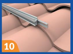
Install our Rail splice kits at all connections between two rails. (10 Ft Lb).
