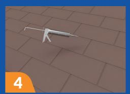
Backfill the pilot hole with Sealant.
