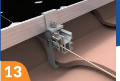
Install the Grounding Lug on each The system is complete. section of rail. Run copper wire to connect them all. Tighten to 3 Ft Lb.
