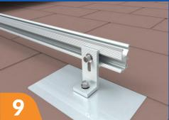
Connect Chiko Solar's proprietary Rail to the L-Foot using a flange nut. Tighten to secure (18 Ft Lb).
