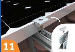
the opening on the top of the rail. opening on the top of the rail. Fasten Fasten and install at all locationswhere at the end of each array (10 Ft Lb). two modules meet (10 Ft Lb). Locations of mid clamps can be determined by panel manufacturer datasheet.
