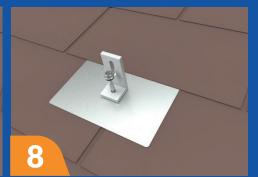
Drive a 3/8" bolt to connect the L-Foot and flashing to the roof (10 Ft Lb).
